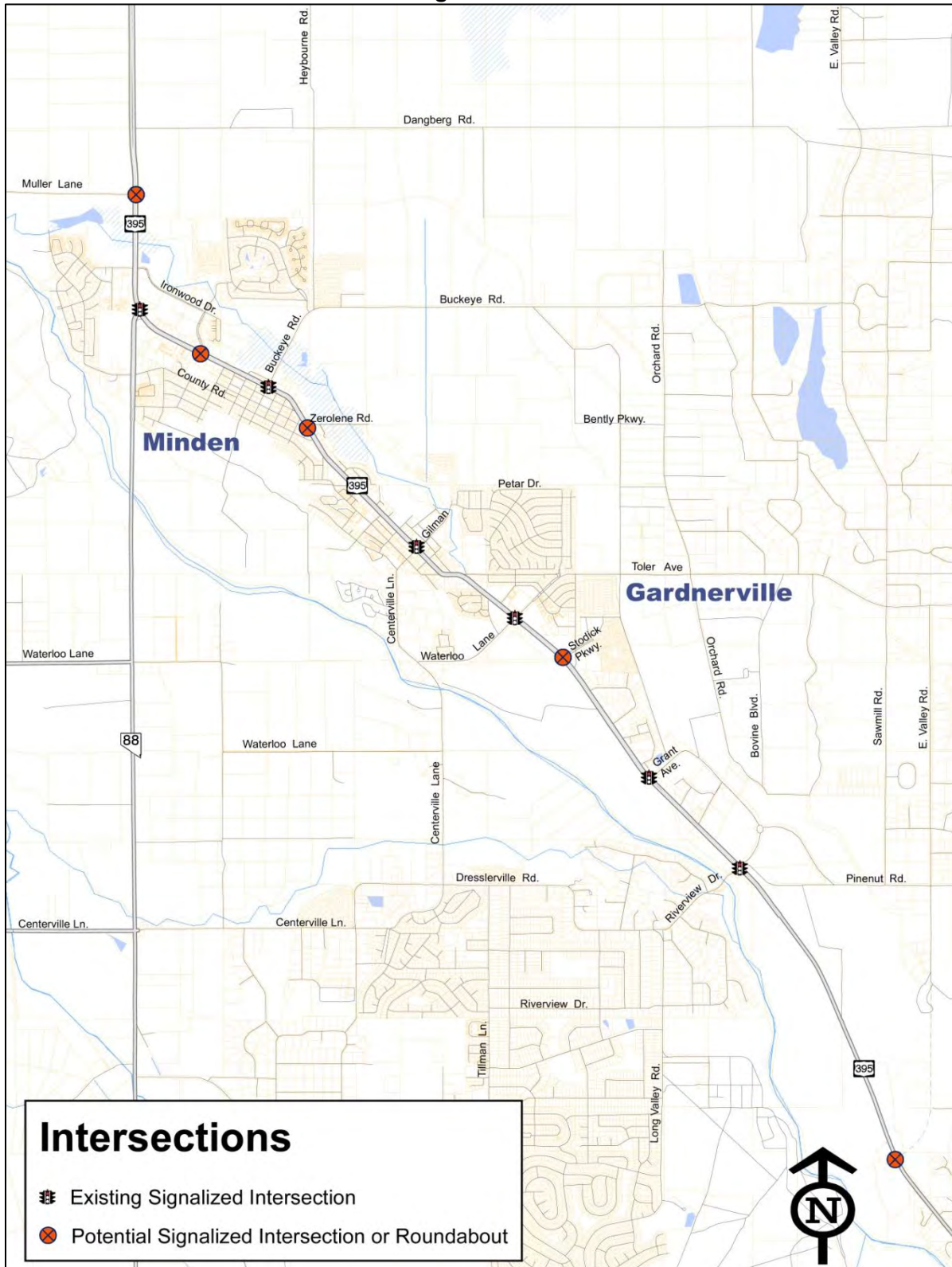
Figure 4.4: Existing Traffic Signals and Potential Future Roundabouts or Traffic Signals in the U.S. 395 Corridor
